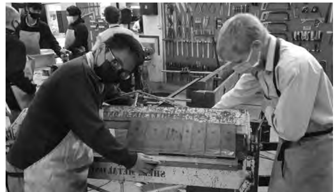
(Pictured, left and right): Ben Ciron and Connor Duffell using the box and pan folder, used for bending the metal.
